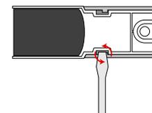
2. Twist away from the clip GENTLY! Until the end cap unclips on the other side.
